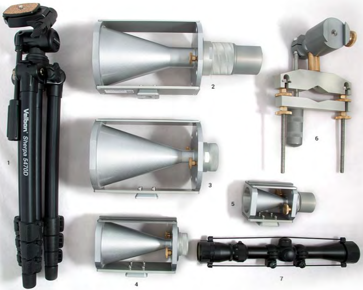
(1) Tripod for antennas (2) Horn antenna 5.9-11GHz (3) Horn antenna 11-17GHz (4) Horn antenna 17-26GHz (5) Horn antenna 26-40GHz (6) Simple pole mount for horn antennas (7) 4x32WR Riflescope for horn antennas
